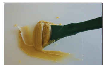
Thoroughly mix DESOWOOD RAP - 4 Hours
